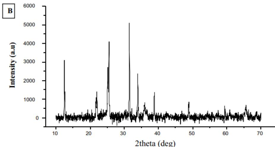
Figure 5: XRD Spectrum of TiO<sub>2</sub> -ZnO at 180 °C
