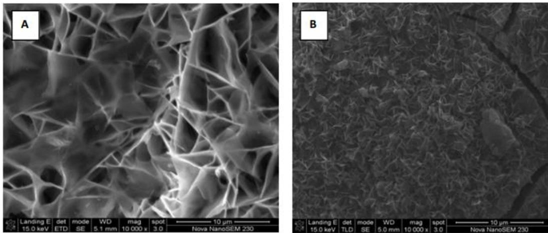
**Figure 6: SEM Images of  $\text{TiO}_2 / \text{Zn}(\text{OOCCH}_3)_2$  Mixtures Prepared at  $90^\circ\text{C}$  at Low Magnification (A) 6hrs (B) 12hrs**
