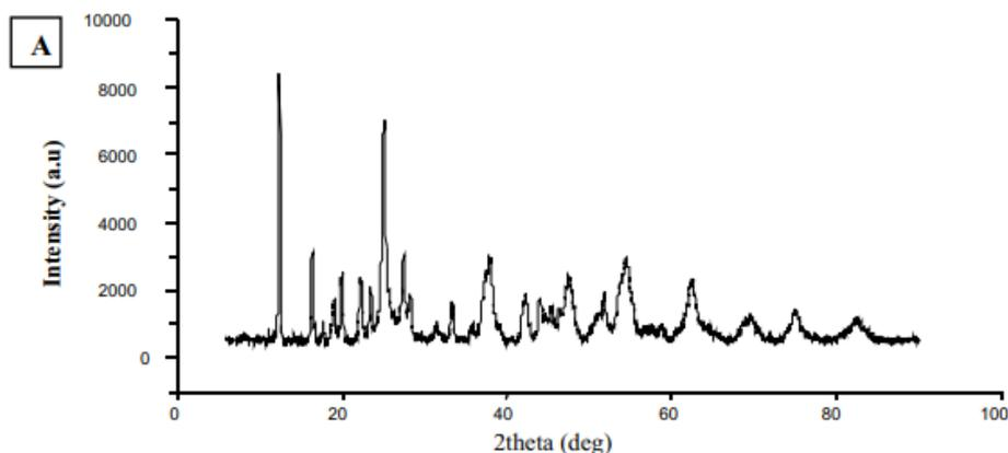
Figure 4: XRD Spectrum of TiO<sub>2</sub>-Zn(OOCCH<sub>3</sub>)<sub>2</sub> at 90°C
