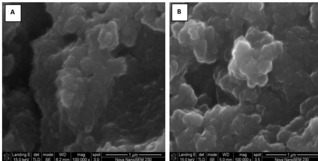
**Figure 7: SEM Images of Representative Product at  $180^\circ\text{C}$  for (A) 6 and (B) 12 hrs**
