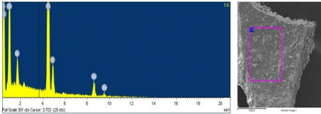
**Figure 2: Spectrum of Energy Dispersion of a Representative Grain**
